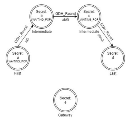
When a GDH\_Round message is received, the first thing to be done is to identify if the current node is an intermediate node or the last node. The current node is the last one if it is the last referenced node in the TSTP class, or if the only node identified after it is the gateway. Otherwise, it is an intermediate node. When the type is identified, it is correctly set.
