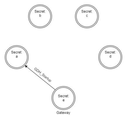
When this message is received, the node adds its own randomized private key to the base point of the chosen elliptic curve. It also sets its type to GDH\_FIRST and its state to GDH\_WAITING\_POP, since it is
