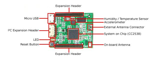
• EPOSMote III pinout:
