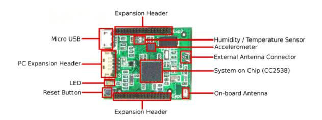
• EPOSMote III pinout:
