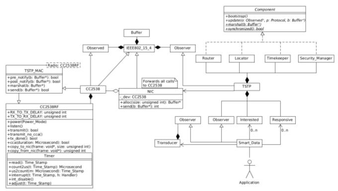
TSTP is a **geographic** protocol, and every node in the network is synchronized in space and time, which means that every node has **spatial coordinates** and a **synchronized clock**. A TSTP network consists of *one* **sink** node and any number of **sensor** nodes. The sink is the reference for clock synchronization and spatial localization.
