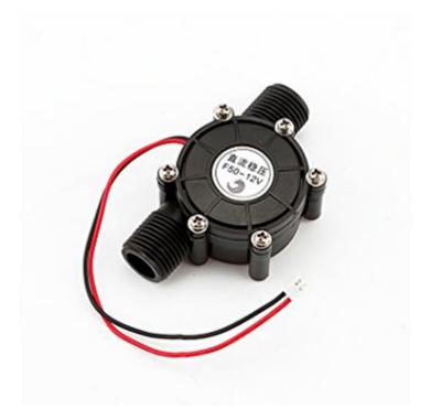
After sensor acquisition, we tested it in an uncontrolled environment to determine the voltage generated by the sensor under conditions of use. The test consisted primarily in creating a flow of water through the sensor, coupling two small pieces of pipe at the ends of the sensor to emulate the building's plumbing, and a voltmeter connected to the output designated to measure the voltage generated. Based on our tests we reached a minimum voltage of 0.2v and a maximum voltage of 12v.
