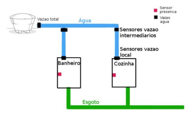
The principle of operation of the model is given by comparing the water flows between the sensor present at the water outlet of the building and the sensors at the points of use (bathrooms, kitchens, etc.). Based on this comparison we can reach the following senarios:
