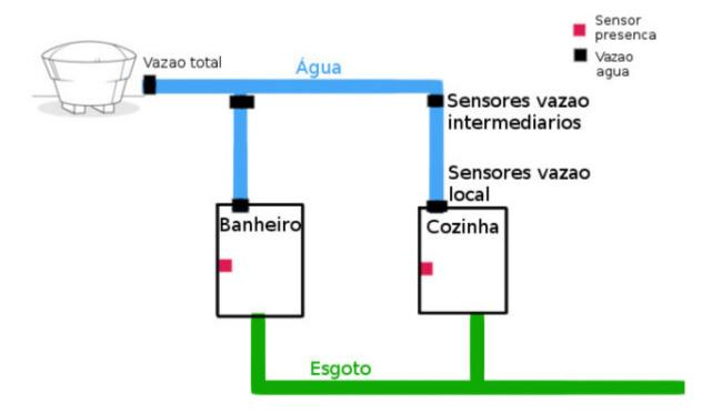
The principle of operation of the model is given by comparing the water flows between the sensor present at the water outlet of the building and the sensors at the points of use (bathrooms, kitchens, etc.). Based on this comparison we can reach the following senarios:
